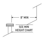
Note: Vents larger than 12" must exhuast a minimum of 12" higher than any part of the roof within 10'
